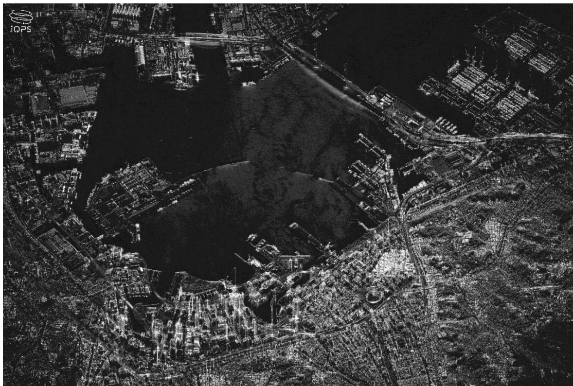
SAR image (Resolution: 0.46m) acquired by small SAR satellite, QPS-SAR-6 “AMATERU-III” at Yokohama City, Kanagawa, Japan
