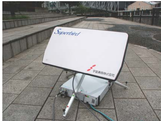
Appearance of the Portalink VSAT
