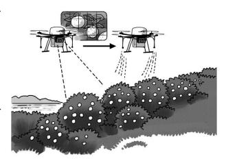
artificial intelligence will immediately determine the pesticide, fertilizer or other chemical agent required, and the drone will then automatically spray crops in the most efficient way. That is what enRoute aims to realize.
