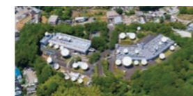
Primary Satellite Control Center – Yokohama Satellite Control Center: Numerous parabolic antennas pointing to satellites from 85E to 169E longitude. Large antennas over 4m in diameter total to 29*3
