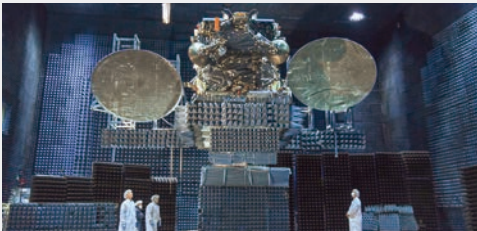
JCSAT-110A Satellite Test ©Space Systems Loral
