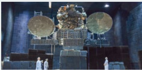
JCSAT-110A Satellite Test ©Space Systems Loral
